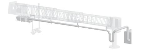
The special construction with flexible outside and inside bearings guarantees a proper adaption of the telescopic tube to axial and lateral movements of the boarding bridge and is furthermore self-supporting over long spans. The gasket designed by IST withstands temperature fluctuations from -40°C to +80°C and is absolutely wear resistant.
